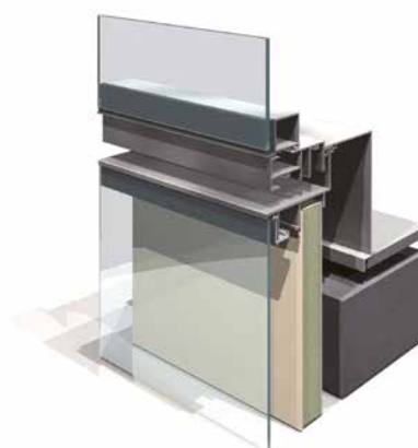
Back panel of Glass Curtain Wall System
