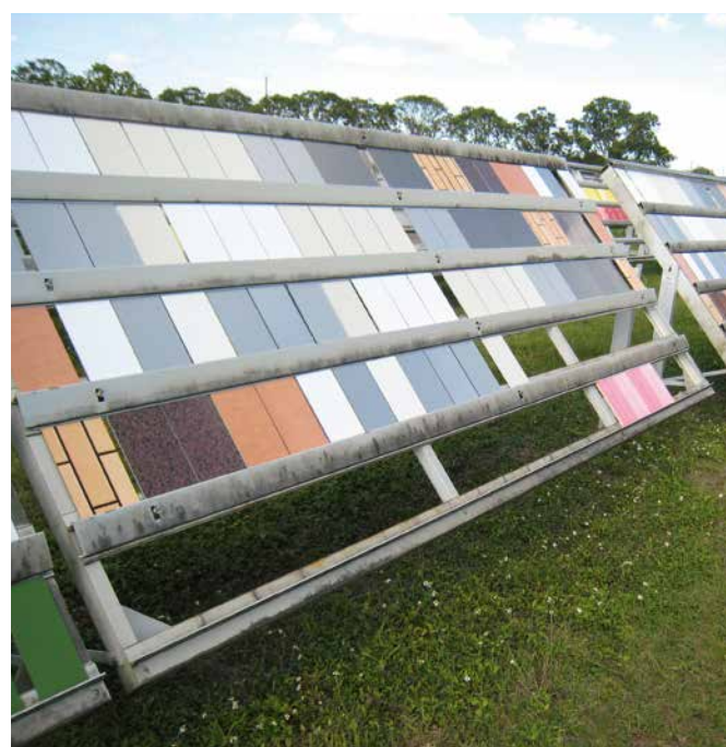
Natural exposure test in Florida, USA
